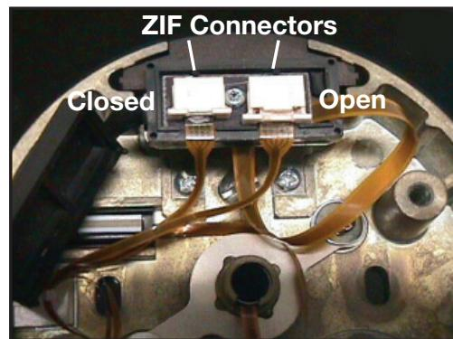
Figure 13 - Closed & Open ZIF Connectors
