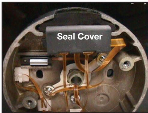
Figure 12 - Open ZIF Seal Cover
