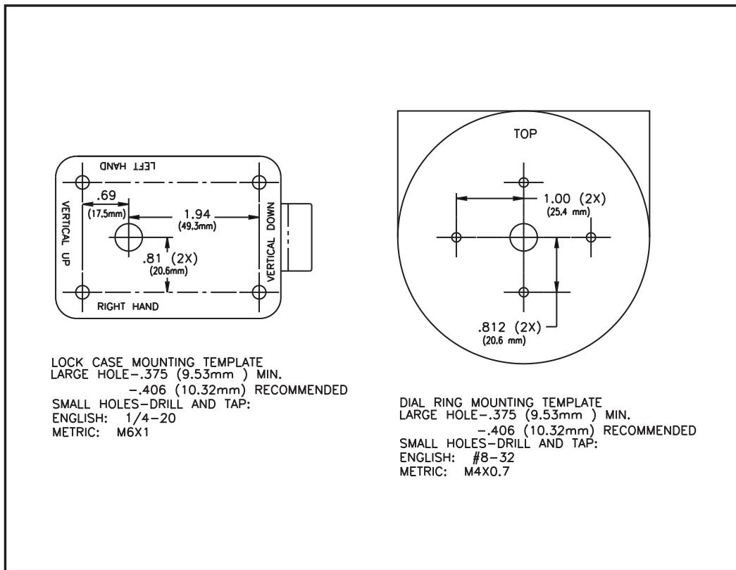
**Note:** The above template is NOT Actual Size. Do Not Use for locating, drilling, and tapping the lock. A Template of actual size is included with the lock for installation purposes.
