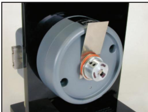
Figure 24 - Place Gauge Between Dial Hub & Bushing
