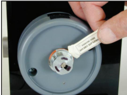
Figure 27 - Apply Lubricant to Ret. Ring
