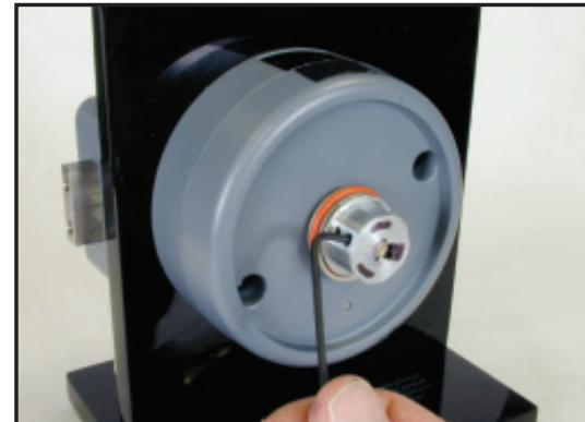
Figure 26 - Tighten Setscrews
