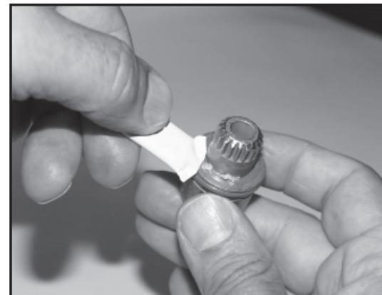
Figure 23 - Apply Lubricant to Hub
