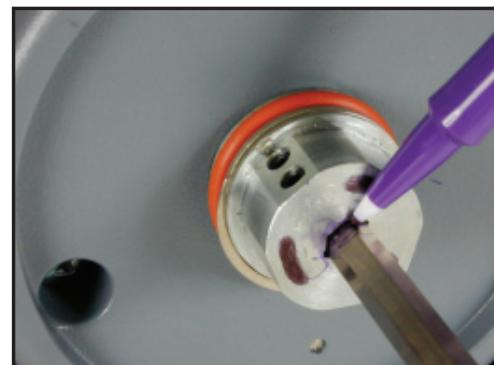
Figure 21 - Mark Spindle Flush to Hub
