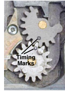
Figure 6 - Do Not Remove Metal Gears
