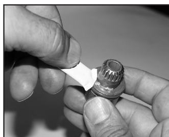
Apply Lubricant to Hub
