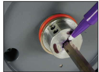
Mark Spindle Flush to Hub
